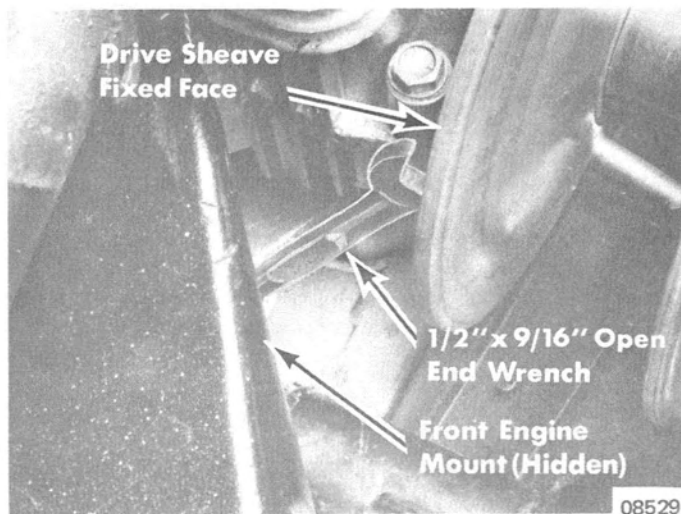
Figure 3. Holding Drive Sheave
